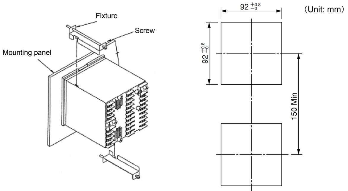
Figure1 Installation method and panel cutting dimensions
