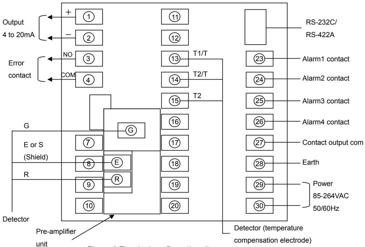
Figure 3 Terminal configuration diagram
