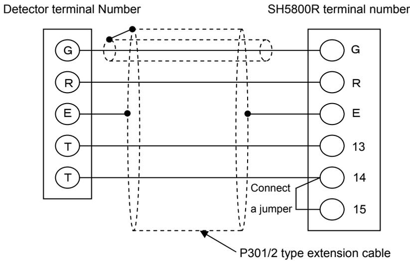
Figure 6 Connection with the terminal box type detector
