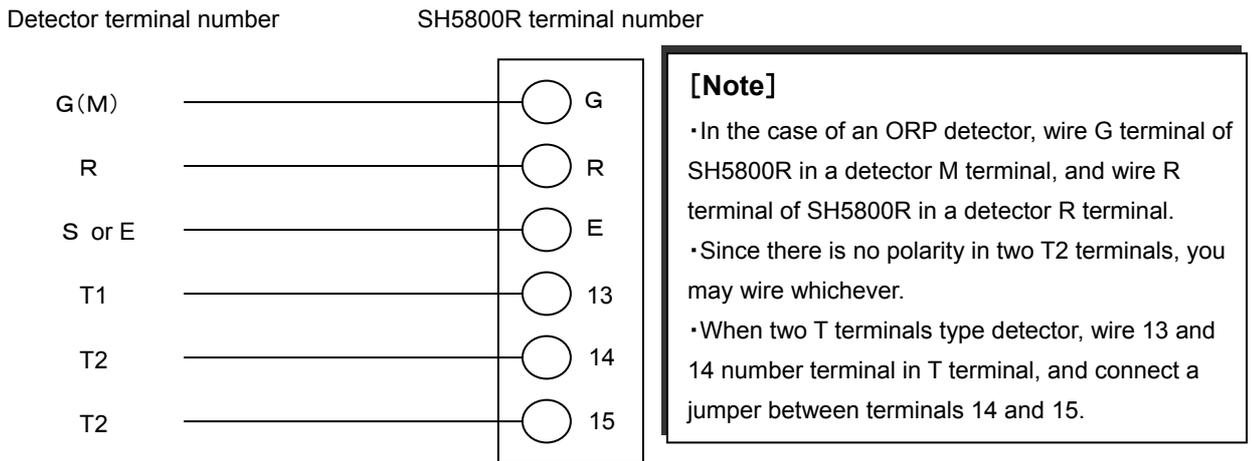
Figure 4 Connection with the cable type detector
