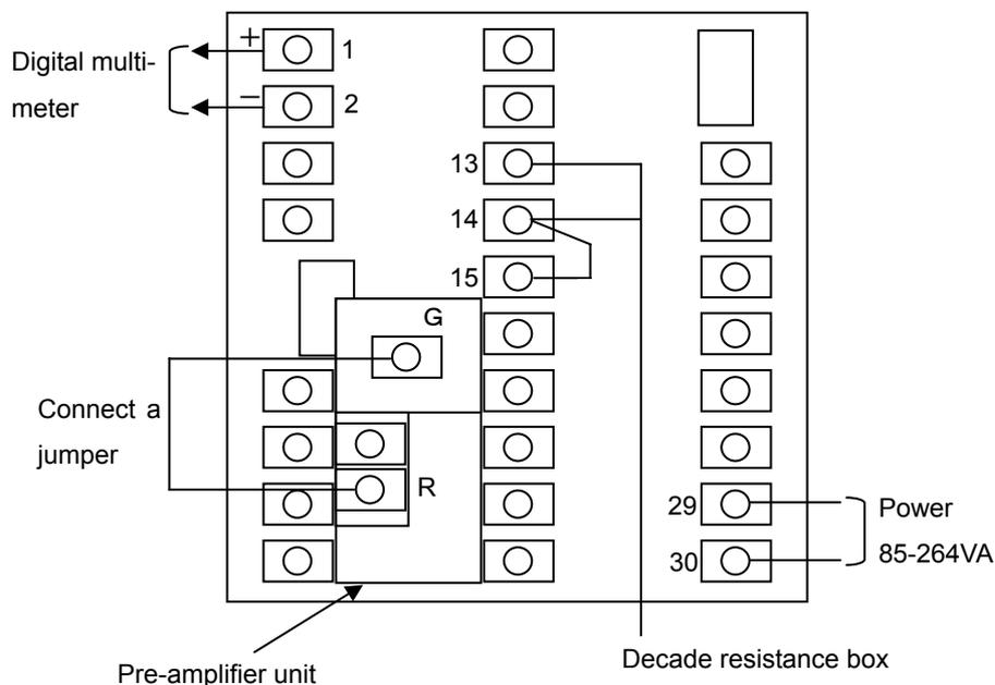
Figure 8 Wiring for maintenance
