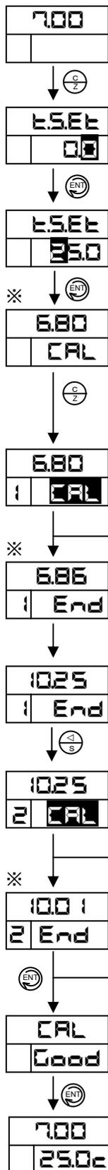
Press the “CAL/ZERO” key for approximately five seconds in the operation mode then the display moves to buffer calibration mode.
