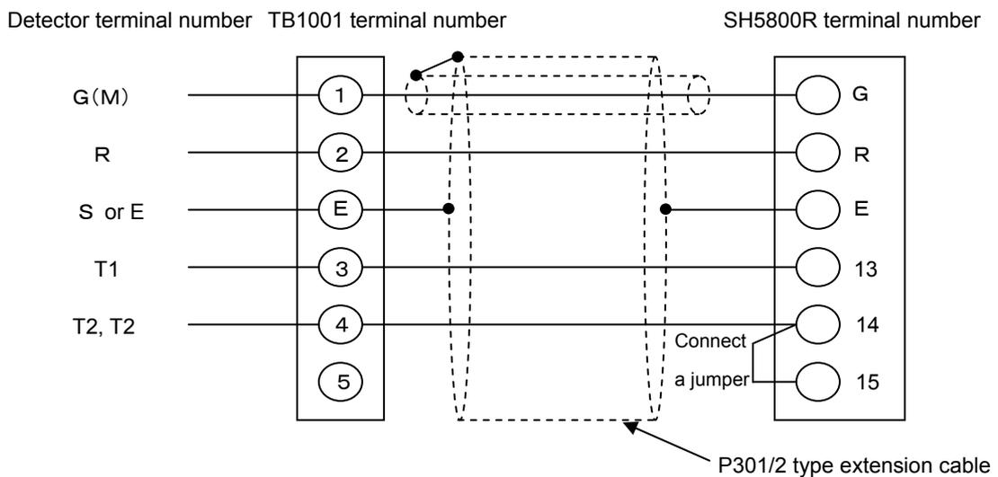
Figure 5 Connection with the cable type detector (2)
